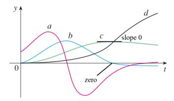
The b-curve is the derivative of the c-curve because the b-curve is zero where the c-curve has zero slope.
