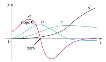
Therefore, the d-curve is the position, the c-curve is the velocity, the b-curve is the acceleration, and the a-curve is the jerk.
